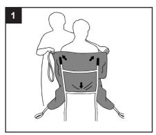
Make sure the positioning straps and sling identification label are on the outside of the sling. Feed the sling down the back of the patient, leaving the aperture at the base of the spine. Check the sling is square across the shoulders.
