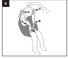
Move the hoist into position and attach the leg straps to the front hooks on the spreader. Next attach the shoulder straps to maintain an upright seated position. The lift may move towards the patient as you do this. When reseating the client, use the sling positioning handles to help achieve a safe and comfortable position.
