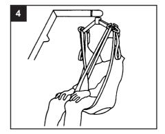
Ensure the sling remains comfortable under the legs and raise the hoist slightly if required before attaching the shoulder straps to maintain an upright seated position. The hoist may move towards the client as you do this. When reseating the client, use the sling positioning handles to help achieve a safe and comfortable position.
