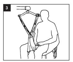
Move the hoist into position before crossing over the leg straps and attaching to the hoist on the front hooks of the spreader bar. An integrated modesty loop on the leg section is also available for increased patient dignity.
